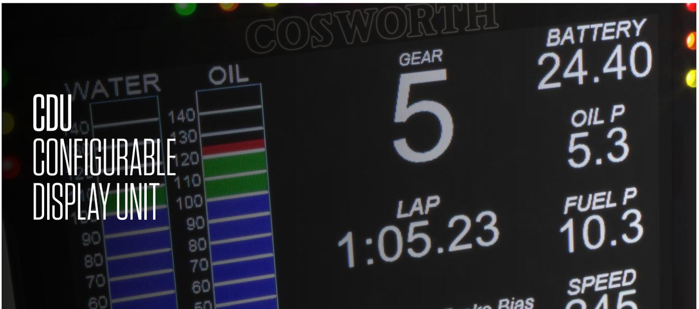
Cosworth's CDU is a fully configurable, compact, lightweight, sunlight viewable TFT display; designed specifically for professional racing applications. The CDU 4.3 incorporates a high resolution, sunlight viewable 900nit, 480x272 QVGA, 16M colour 4.3" TFT display, with the CDU 7 incorporating a viewable 2000nit, 800 x 400 QVGA 7" TFT display. Together with 16 fully configurable RGB LEDs, all controlled via Ethernet from a range of Cosworth data loggers and ECUs.
