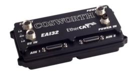
Individual inputs can be software configured as either single ended (up to 32) or true differential (up to 16). Each of the two input connectors also offer four 0-10V programmable excitation lines, two of which can be software configured as switchable outputs.
