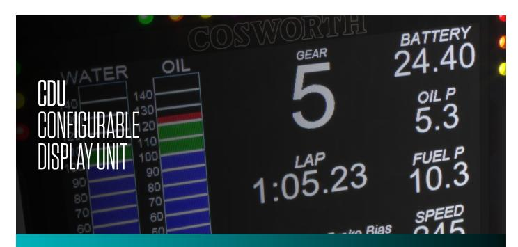
Cosworth's CDU is a fully configurable, compact, lightweight, sunlight viewable TFT display; designed specifically for professional racing applications. The CDU 4.3 incorporates a high resolution, sunlight viewable 900nit, 480x272 QVGA, 16M colour 4.3" TFT display, with the CDU 7 incorporating a viewable 2000nit, 800 x 400 QVGA 7" TFT display. Together with 16 fully configurable RGB LEDs, all controlled via Ethernet from a range of Cosworth data loggers and ECUs.
