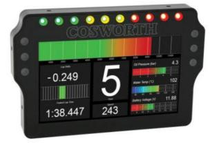
Multiple displays may be daisy chained together and configured to display independent custom pages controlled from a single Cosworth data logger or ECU, e.g. rally driver and co-driver display.
