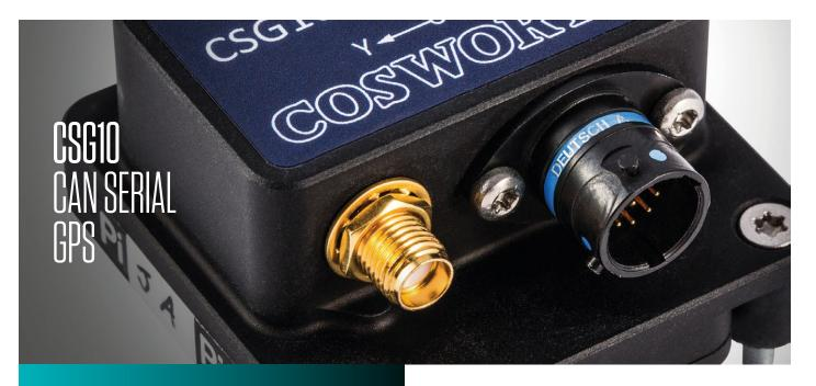
Cosworth's combined GPS and motion pack unit provides market leading positional accuracy and 9-axis motion data in a cost-effective, single-box solution. With rapid start up times, support for the latest satellites and flexible CAN/serial integration, the compact and lightweight unit is perfectly suited for a variety of applications.
