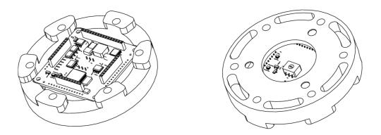
The CSB housing has been designed to allow the CSB to be fitted onto the back of any steering wheel. The spacer has fittings for either a 3 or 6 hole boss.
