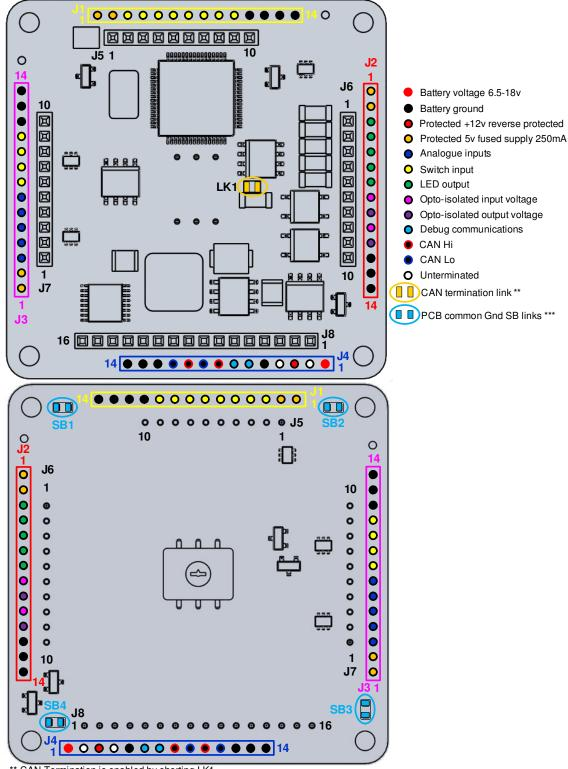
\*\* CAN Termination is enabled by shorting LK1
